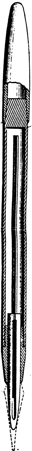
(Face Simile of Cooley Patent Pen—Sectional View. Showing taper cap and joint.) Issued years before the Inventor (?) Waterman's.
